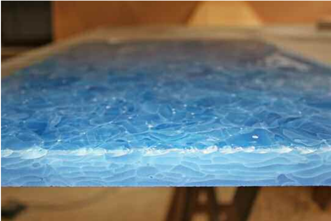
Torn Edge caused by unclean Processing
